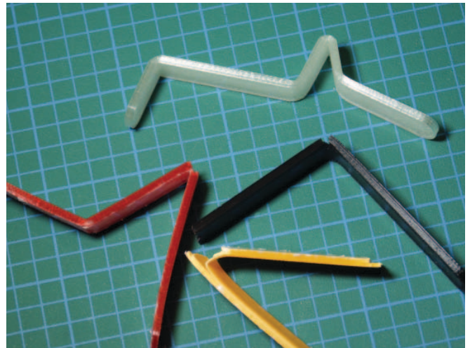
Among the samples that Voxel Factory sent me was an unexpected surprise: ColorFabb XT-Copolyester (top) was the only plastic that I could bend this way and not break. And it proved almost as rigid as polycarbonate. It's definitely one of the better filaments in the PET family.
