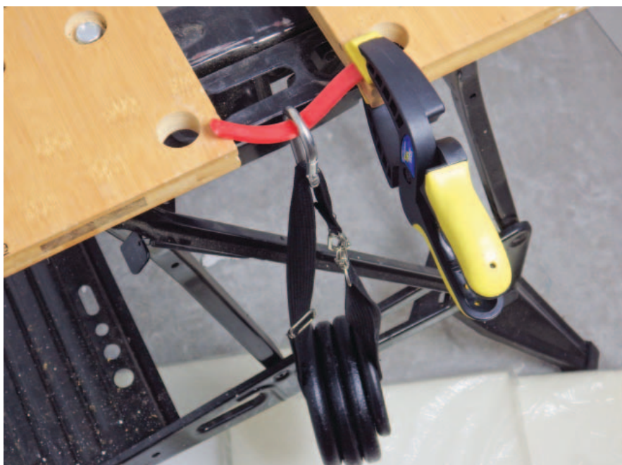
I applied weight at the center of each stick until it failed. This gave me an approximate idea of its rigidity and strength. Hang in there polycarbonate! This is the strongest material that I tested.
