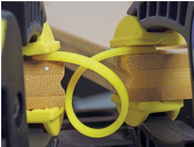
Nylon is the only rigid 3D printing material that can be curled up like this and not break. It did not even lose its shape. I was able to straighten it back afterward.
