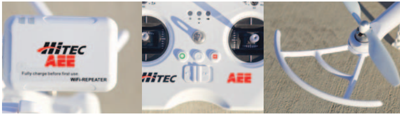
Left: The WiFi-Repeater amplifies the signal from the Q-Cop 450 to your smartphone. Center: The three center buttons control the camera, the left is video start, center is the shutter button and the right is for video stop. Right: The blade guards and props are the only two things to assemble. Far right: Not only do the red and green LED lights help with orientation, but they also signal alerts such as low battery warning.
