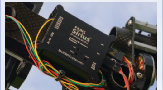
PID CONTROLLER. A PID controller is a control loop feedback mechanism widely used in industrial control systems. It calculates an error value as the difference between a measured process variable and a desired setpoint. Its algorithm involves three separate constant parameters: the Proportional, the Integral, and Derivative values. The "P" is the amount of correction, "I" adjusts how fast the correction occurs, and "D" adjusts how much change is allowed to occur based on past changes. The weighted sum of these three actions is used to adjust the process via a control element, such as the position of the camera.
