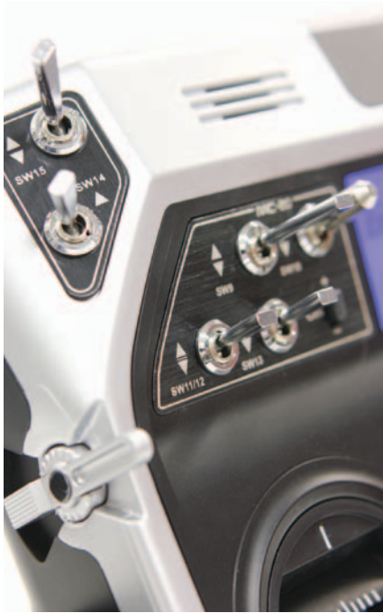
Note the speaker grille: it emits audible telemetry readouts, warnings, and even music!
