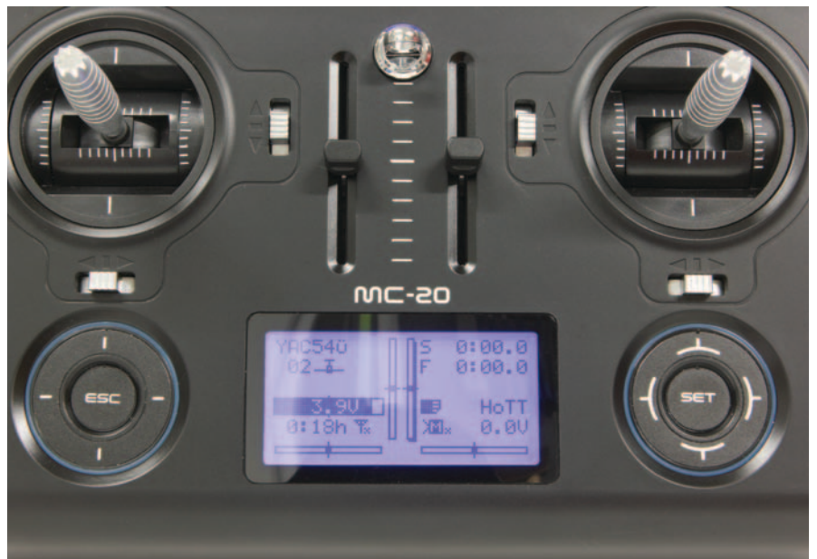
Touch pads navigate through menus, backlit screens are easy to view, and we love the center slide trims in addition to the digital ones.
