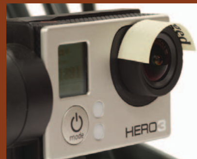
Even something simple like this business card stock taped down on the lens will work as a hood.
