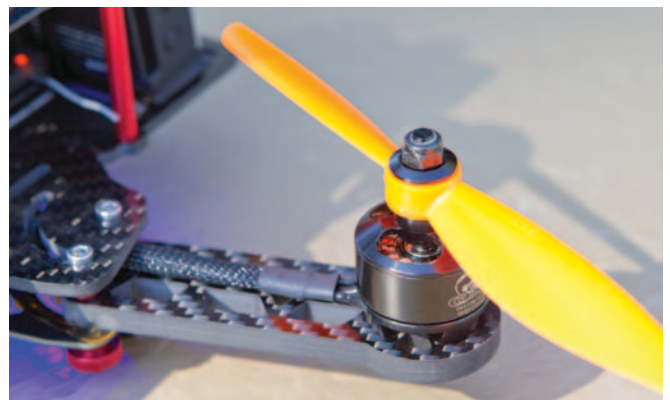
Because both the motors and arms are really stout, you can take a surprising number of direct hits before they need to be replaced.
