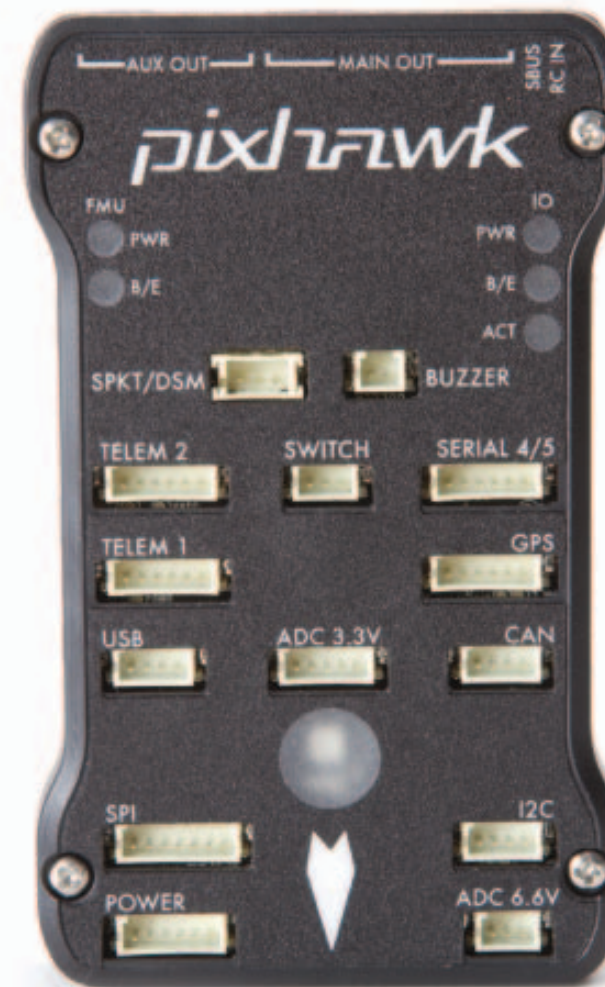
Pixhawk's flight controller has many telemetry plugs, which allow pilots to customize the telemetry features that they want to receive from the multirotor.
