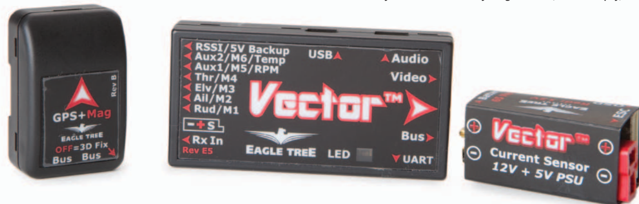
Eagle Tree's Vector flight-control system utilizes GPS and has many telemetry features that are easy to add on. It also has a fully configurable OSD (on-screen display) built in.
