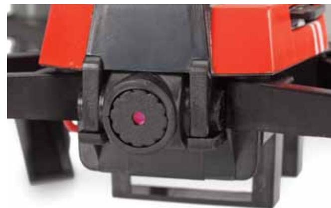
Below: The built-in camera is controlled with transmitter buttons and a touchscreen, using the downloadable app. The lens can be manually adjusted for view angle.
