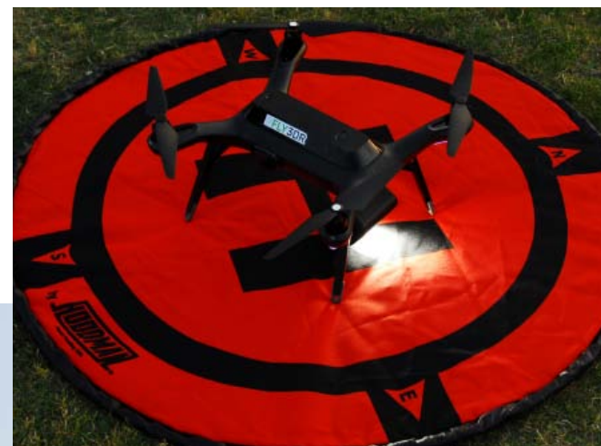
The 3DR Solo/Fiilex AL250 configuration is ready to take flight from a Hoodman Launch Pad.
